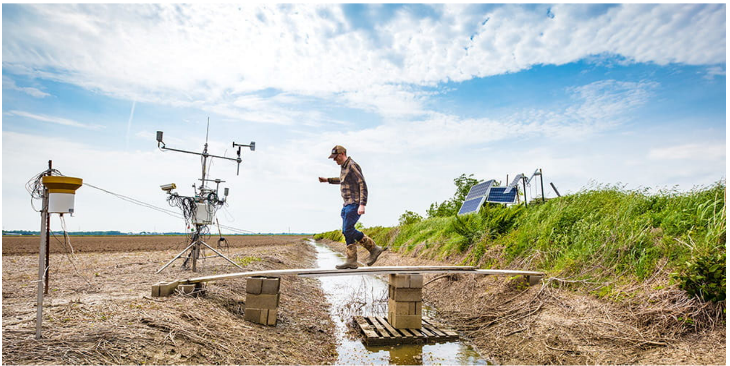
Dr. Benjamin Runkle at Chris Isbell's rice field, three miles south of Bayou Meto conducting research on reducing Rice's Carbon Footprint. The tower, 12-feet tall and supported by tripod sticks, measures everything – the basic, such as air temperature, rainfall, wind speed and relative humidity, and the advanced, including soil nutrients and acidity, water vapor concentration, water evaporation rate, soil moisture and temperature, and, perhaps most importantly, carbon emissions in form of methane and carbon dioxide.
