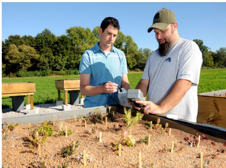
Green roof study — Biological engineer Brian Haggard, top left, and graduate student Channon Toland test chemical content in runoff water from a mock green roof at the University of Arkansas Division of Agriculture's Watershed Research and Education Center. The study is a joint research project of the Division of Agriculture and the UA, Fayetteville, School of Architecture's landscape architecture program.
